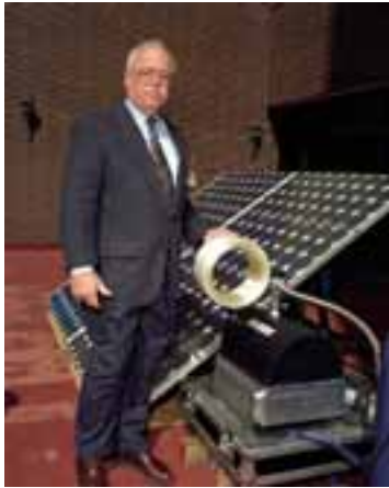
Flywheel technology is one possible technology for storing energy. It is based on transferring the energy to a kinetic battery spinning at very high speeds. When the flywheel is slowed, the energy is released.
